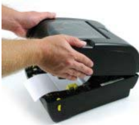
Figure 9: Use both hands to close the top cover
